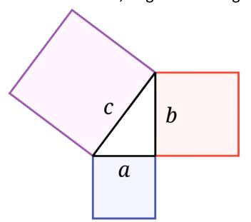
We can rearrange this theorem to find the length of any of a given triangle's sides so long as we are given the length of any two of its sides. For example, to find side *a*, we can rearrange the equation like this:  $a = \sqrt{c^2 - b^2}$ .
